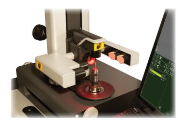
First front camera allows to measure and inspect tools with 26X magnification with the possibility to have 2X and 4X digital zoom.
