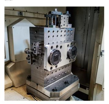
For a long time, no standardized palletizing system was used to set up and reset electrodes and workpieces on milling and EDM machines. Setting up times were correspondingly considerable. Depending on the job in hand, machines had downtimes of several hours.
