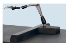
Using the dial indicator on a flexible base, align workpieces in the Z-plane or the Y-axis along the stop guide rail.
