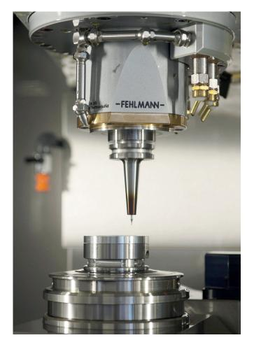
During set-up, the brass blank to be machined is mounted on an EROWA size 72 holder with mounted fixture. Then the fixture is clamped to the EROWA PowerChuck P on the machine table in no time. The positioning accuracy of the fixture in the chuck is <0.002 mm.
