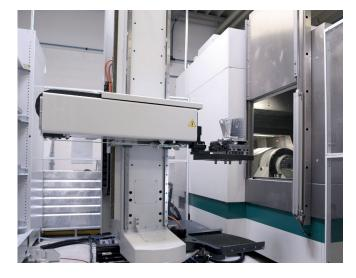
Manufacturing programs are created at Mastercam programming stations and managed in a central database. The Versa is networked with the whole system. The EROWA JMS 4.0 ProductionLine process control system then delivers a smooth production workflow on the machine. The software controls and monitors the machine and robot and manages the various jobs.
