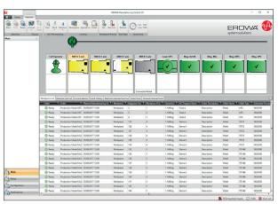
Job data I Information on the effective machining time for each workpiece or for the entire job.
