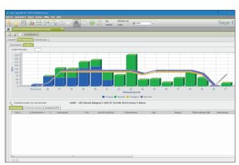
**MES I** The production planning system fetches the master data from the ERP, and adds planning details such as machine assignment and standard times.
