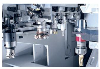
If a tool is missing or if its life has expired, its sibling tool is used instead. If none is available, the current job is stopped, and the next job on the priority list is processed.
