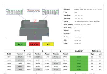
The measurement logs can also be stored as 3D PDF files, providing a graphical view of the verified measuring points.
