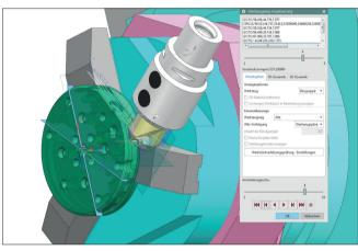
**CAM I** CAD data is imported via the interface to CAM. CNC programs are generated and provided ready for use.
