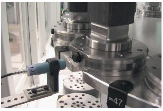
Staged pallets with workpieces are uniquely marked with a chip. At every station in the production process, each pallet is precisely identified by the EROWA EWIS™ system.
