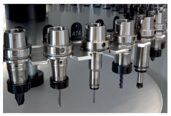
The ToolManagement module checks which tools are required based on the NC program right after a job has been created. A comparison with the tool list of the machine shows whether the job can be released or not.
