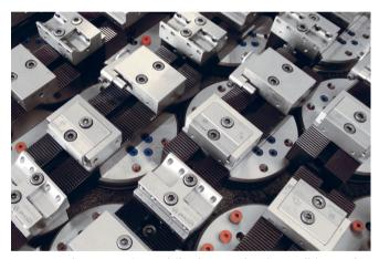
Setup and preparation while the production cell is producing. There is no waiting time. The EWIS™ chip ensures identification.
