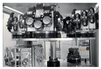
Fixture Manager manages multiple fixtures on a pallet, automatically storing the position of a clamped workpiece. The identification system ensures the correct matching of the data.
