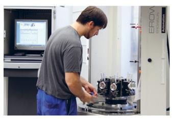
Finished parts are automatically routed to the tooling station. Clamping new blanks is supported graphically.
