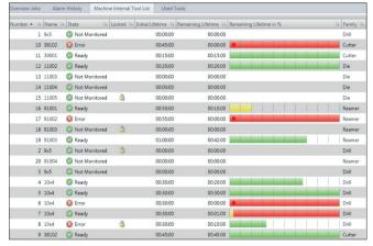
Clear presentation of the tools at the machine including status, tool life, tool breakage and a forecast of the available production time with the existing tools.
