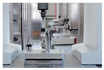
The "washing/cleaning" production step is necessary if several processes run in succession automatically. E.g. mill > wash > measure workpiece.
