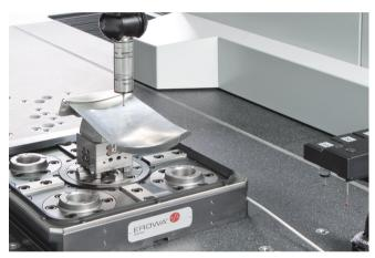
**CMM Qi I** Datum points are identified easily at the measuring station. The data is associated with the workpieces via the integrated interface.
