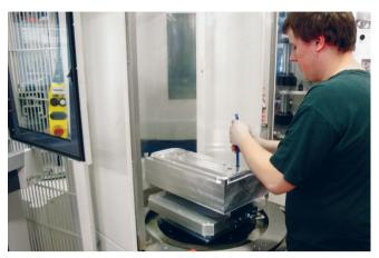
More workpieces are prepared while the machine is in production.
