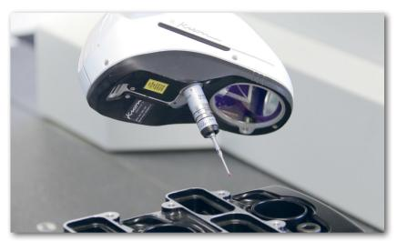
During "normal measuring", only individual points are measured. With scanning, large data volumes are captured. This results in substantially more detailed information about the form and shape of the workpiece.
