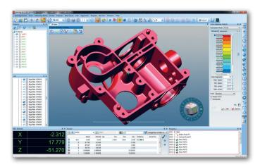
Simple CAD import function which is also able to process large data sets without any problems.
