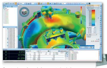
Easy-to-view color-coded representation (color mapping) for an intuitive inspection of dimensional accuracy.
