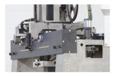
The centrally positioned axis drives allow symmetrical movements on both sides.
