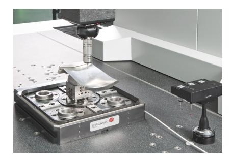
During "normal measuring", only individual points are measured. With scanning, a large amount of data is recorded. This generates much more detailed information about the form and shape of the workpiece.
