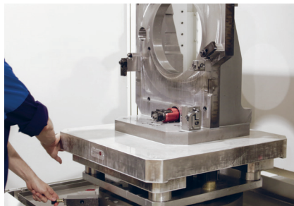
Preparing for automation: fixture with MTS interface.
