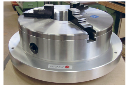
MTS pallet ø 400 mm with 3-jaw chuck.
