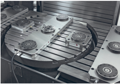
Machine table with flexible MTS clamping options.
