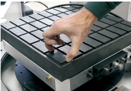
Vacuum clamping on an MTS pallet.
