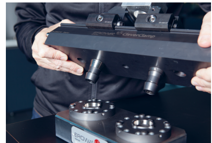
MTS 81 base plates offer flexible clamping options requiring minimal space.
