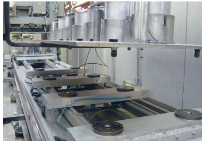
Customized table equipment with large MTS pallet.
